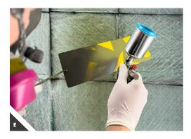
• Flash Cure at 150-180°F (65-82°C) for 10 to 30 minutes, or just to the point of tack-free (dry to the touch). Allow the items to cool to room temperature before moving to the next step.
