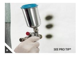
**PRO TIP**: IWATA LPH80 baseline settings for achieving a 1" oval fan pattern with moderate splatter.
